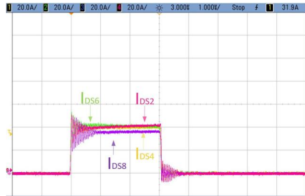
Figure 4.8: Current sharing of the SiC MOSFETs. Measured drain current of each SiC power module.
