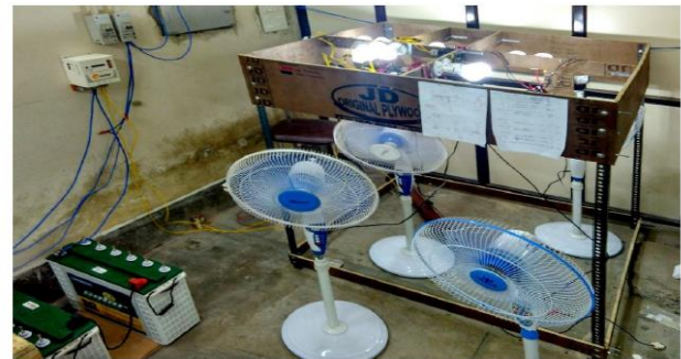
Figure 8: Hardware implementation of the DC house
