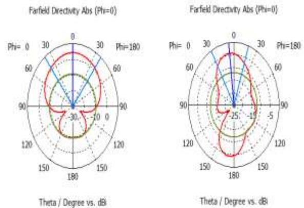
Fig.5: Polar plot of directivity for phi and patch antenna
