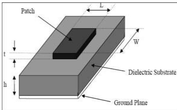
Fig.4: Microstrip Patch Antenna
