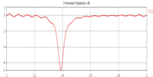
Figure 1: RL curve of an antenna
