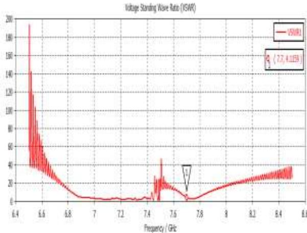
Fig. 11: VSWR Curve of EBG Structure of Patch Antenna
