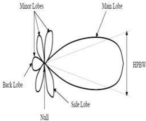
Fig.3: radiation pattern of HPBW from
