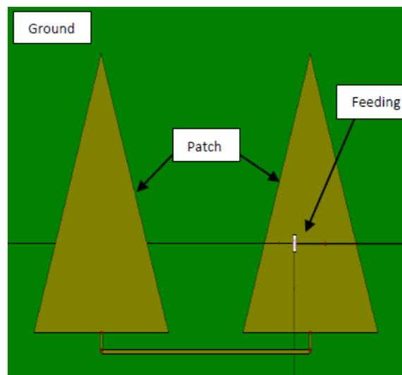
Fig.2: Patch element antenna array
