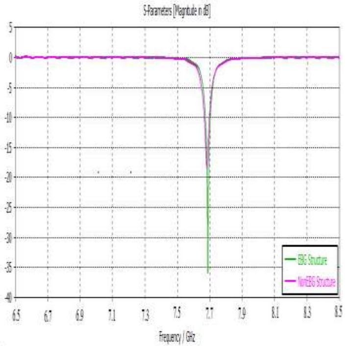
Fig.9: Reflection Loss curve Patch antenna and EBG without EBG structure antenna
